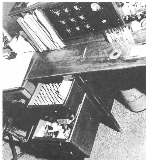
Wires led from patient to ammeter next to dials of Drown Diagnostic Machine. Operator rubbed finger on pad (right) beside hole in which were set vials from drawers.
